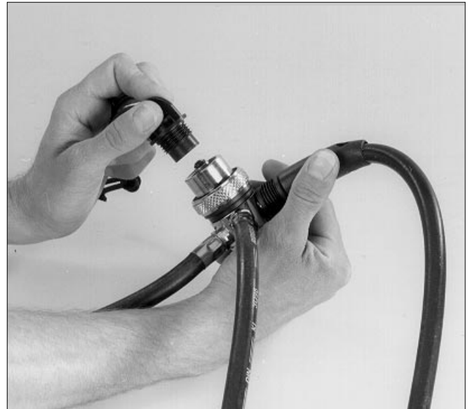
Fig. 6.20 Mounting of protective cap at pressure reducer
