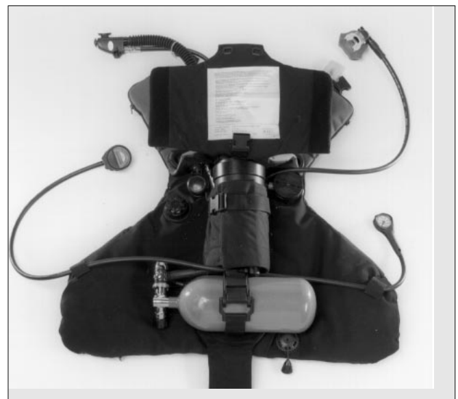
Fig. 6.17 Securing of the CO 2 -scrubber cartridge
