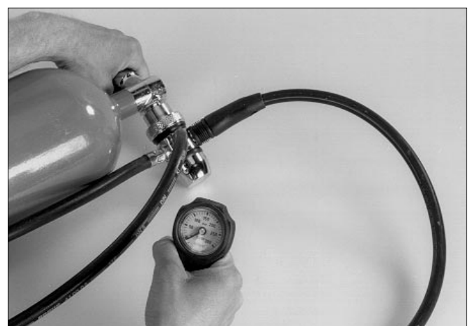
Fig. 6.18 Checking cylinder pressure
