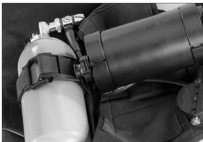
Fig. 6.15 Connection of the sodalime cartridge
