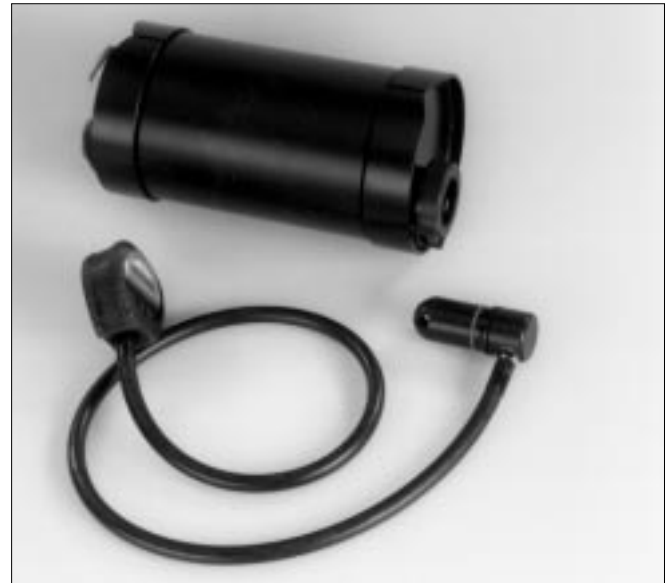
Fig. 6.16 Connection of Dräger Oxygauge
