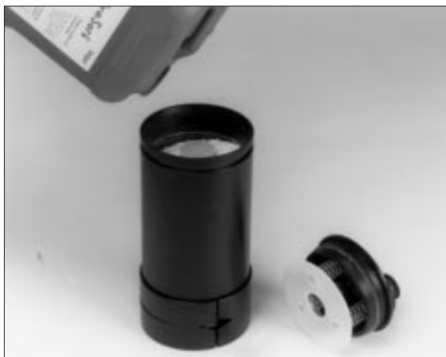
Fig. 6.8 Filling the cartridge with sodalime
