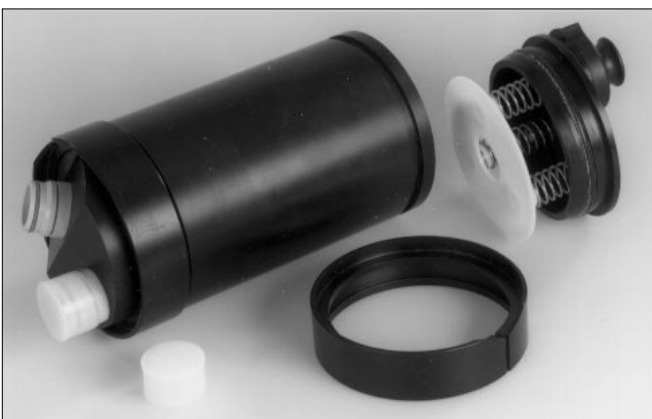
Fig. 6.7 Removal of bottom cartridge lid
